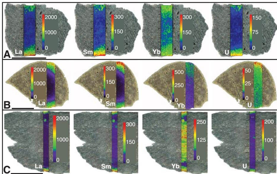
**Figure 1.** Laser ablation–inductively coupled plasma–mass spectrometry maps of distribution of light (La), middle (Sm), and heavy (Yb) rare earth elements (REEs) and U in bones from bonebed in Cretaceous Judith River Formation, Montana, USA. Numeric scale in parts per million. **A, B:** Bones show concentration gradients in all elements. **C:** Bone shows concentration gradients at outer margins and enhanced uptake of heavy REEs within center of bone. Scale bars = 5 mm.
